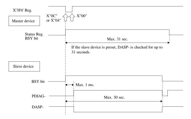
Figure 6.3 Response to software reset
